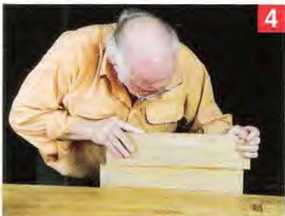
Hold the top board so you can bear down on it with your weight while rubbing it a few inches back and forth to force excess glue out.
