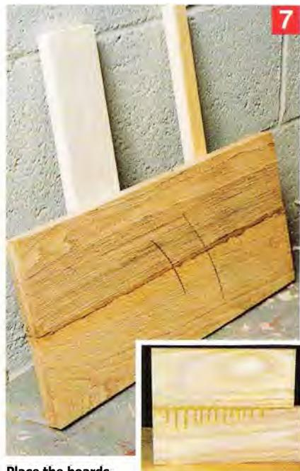
Place the boards out of the way while the glue cures overnight. The heavy-handed glue application on my practice joint (inset) indicates that it has been a long time since I made a rub joint!
