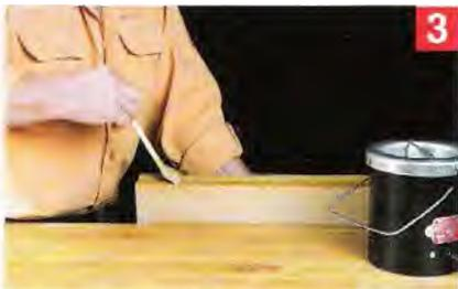
With one board held in the vise, hold the second to it by hand as though they were hinged. Spread glue evenly and thinly to wet both faces.
