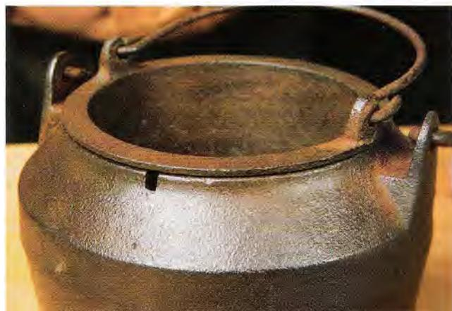
My benchmate from college days sent me this tired glue kettle from the U.K. It's smaller than any I used and unusual in that the glue pat is flat-bottomed. Every one that I used had a hemispherical bottom **Eft**\* deterred users from removing it from its hot water bath. I'm sure steam vent in the kettle casting was marketed as an "advance" iv Ole kettle technology.
