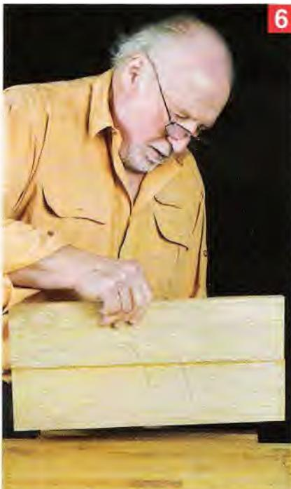
Within a minute or two, the glue has cooled sufficiently to allow you to lift the boards out of the vise.
