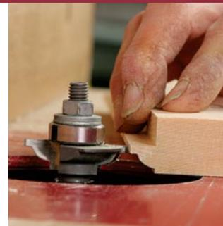
**Use a test block to set the bit height precisely.** A single test block aligns the bit that cuts the stick profile (photo left) and the bit that cuts the cope profile (photo above).
