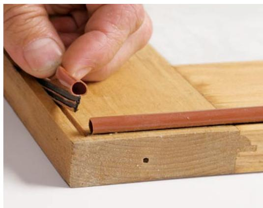
**Weatherstripping: where energy efficiency and tradition meet.** Barbed weatherstripping beads are available through Resource Conservation Technology Inc. (410-366-1146). I cut a groove with a standard 7/8-in. straight bit in a router, then push the barbed bead into the slot with a J-roller.
