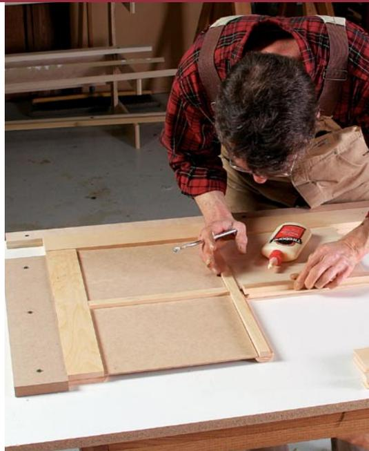
**Cope-and-stick profiles provide lots of glue area.** On this 7/8-in.-thick stock, there's 1 1/2 in. of surface area for the glue joint.
