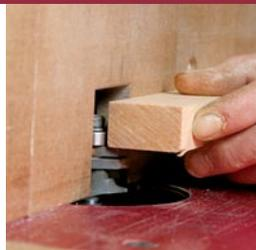
**Align the guide bearing with the fence.** The guide bearing acts as a depth gauge for the fence position. If the bearing protrudes from the plane of the fence, a bump or burn cut can result.
