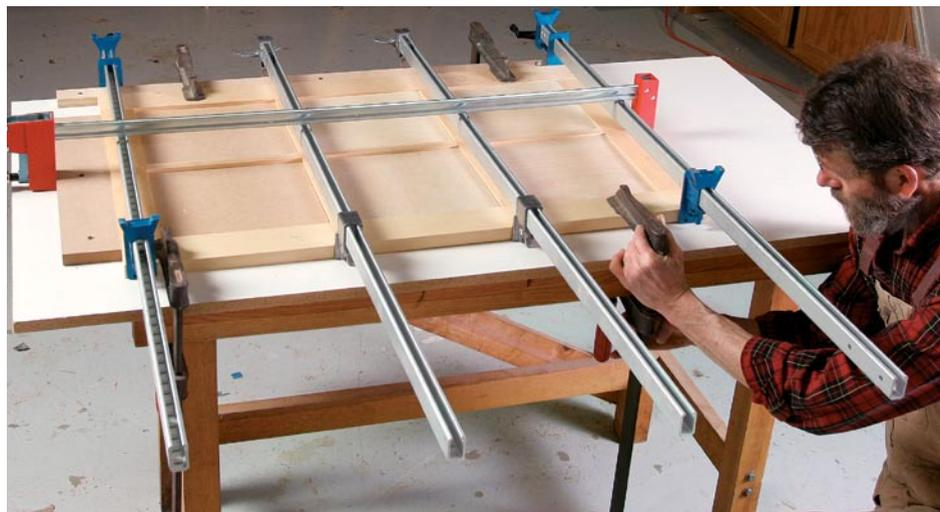
**Pull it all together, and keep the frame flat.** Set the bar clamps in place and loosely tightened, pull the frame flat to the table with clamps at the corners, then tighten the bar clamps and corner clamps in unison.
