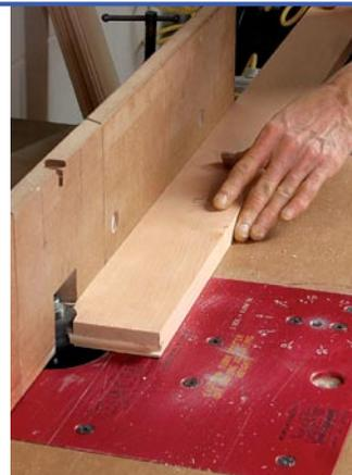
**Remove tearout with the stick bit.** The window stiles are wide enough to be guided safely by hand against the router fence.
