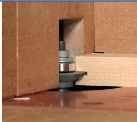
**Keep the stock running square to the router-table fence.** By coping the ends first, I can remove tearout on the next pass with the stick bit. If your router table has a miter-gauge slot, you can guide the workpiece with a miter gauge. Otherwise, use a guide block.
