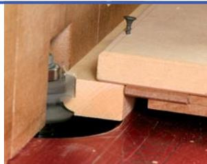
**Use a safety sled to rout muntins.** These narrow parts can't be guided safely by hand. This sled (left) holds the workpiece securely while allowing my hands to stay well clear of the bit.
