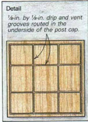
Box newel post is composed of four 1-in. thick cedar boards biscuit-joined and glued together, all of which slips over a pressure-treated 4x4.
