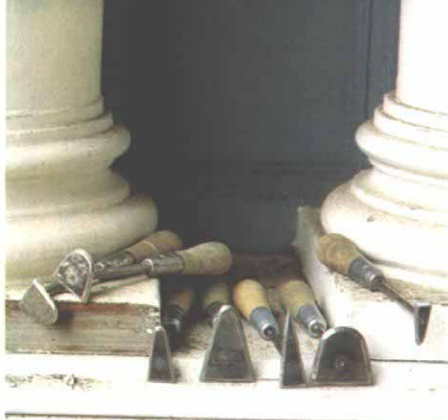
Painters need a variety of scrapers to correspond with the nooks and crannies that distinguish Victorian detailing.
