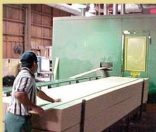
**M**DF is made of a wood-fiber and resin mixture that's compressed into long, flat sheets. After the sheets are ripped into appropriate widths, they're run through a molding machine to form the profile. High-density MDF trim is a smart choice in high-traffic locations and for long, straight runs. Lower-density products are lighter weight, but they aren't as durable and don't hold fasteners as well. Many local and regional lumberyards purchase or mill their own MDF
