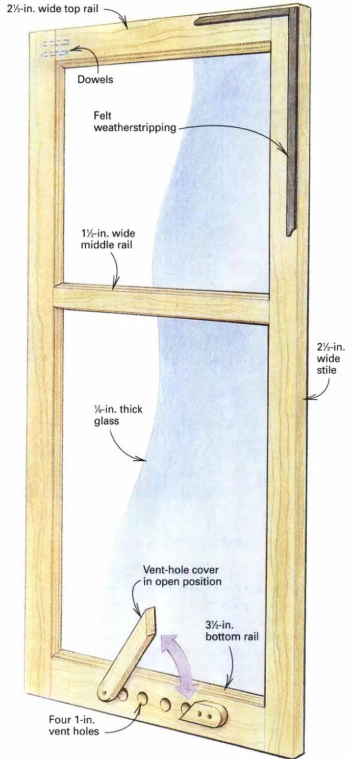
lot of stress, they would be moved around. That movement, combined with the weight of the two large panes of  $\frac{1}{8}$ -in. glass they would bear, made doweled joints my choice.
