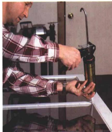
**Polyurethane glazing caulk means fast glazing.** After the glazier pointed the glass in place, he glazed the window in minutes using a caulk gun and a tube of polyurethane window-glass caulk.
