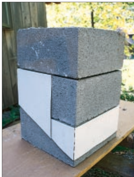
Figure 6. In this mock-up, the V-shaped leg of both the upper and lower pieces of counterflashing is locked into the joint between chimney blocks. A bead of caulk in the joint will keep out excess water and wind-driven rain.
