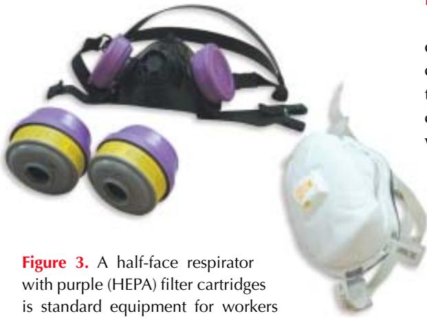
**Figure 3.** A half-face respirator with purple (HEPA) filter cartridges is standard equipment for workers who routinely disturb lead paint (the extra-thick purple and yellow cartridges offer additional protection from lead or chemical fumes). Remodelers, electricians, and other workers who don’t disturb lead very often can wear a comfortable N100 disposable respirator.
