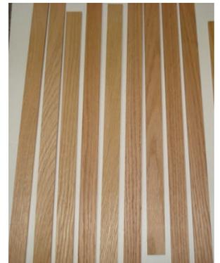
Cut several extra strips as the little nibs can break off in the process. Don't cut your strips to length until after you have assembled them.
