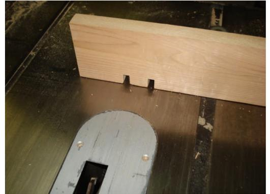
Place a little piece of your strips in the slot. I made mine long so I could cut five strips at once. Wax the saw top and sliding miter gauge so everything moves smoothly.
