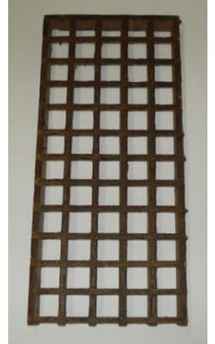
You need a dado blade on your table saw. An adjustable one is ideal but if you do not have one pick a combination of dado blades about a quarter of an inch thick and then cut your strips that exact thickness.
