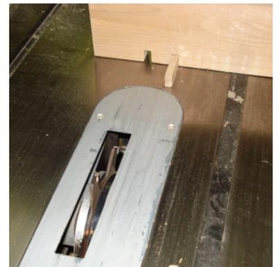
Cut one slot in your strips then move the strips onto the little strip of wood and cut another slot.
