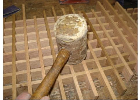
When you are finished assembling, cut the ends of the strips off.
