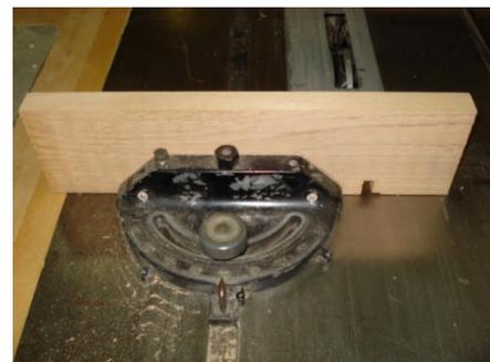
Make an index pencil mark on the wood and miter gauge. Move the wood over the exact width of the planned spaces in your grate. Cut the second slot in the fence. Move the wood back to the index mark and screw it back on again. The blade should be half or more as high as your strips are wide.
