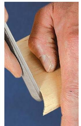
**5** **The back bevel allows minor adjustments** to be accomplished using a few passes with a wood rasp rather than a belt sander.
