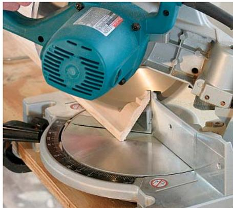
**1** Place the crown molding upside down in the miter saw and at an angle between the fence and base. Then make a 45° cut to reveal the profile for the cope.
