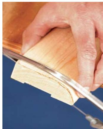
**4** **Angle the blade into the work** so that the face of the cut becomes slightly proud of the back side. This slight angle is called a back bevel, or back cut.
