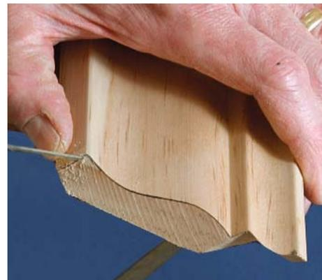
**4** Work inward from both edges to ensure that the last saw stroke separates the meaty center of the molding rather than the fragile outer edge.
