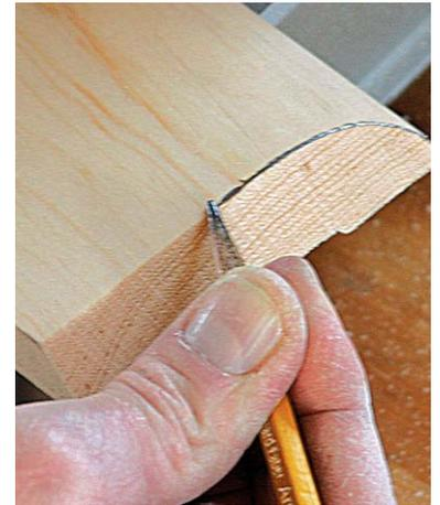
**2** **Use a pencil to highlight the cutline.** To make the profile of the molding more apparent, draw the flat edge of a pencil lead across the inside edge of the miter cut.
