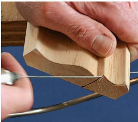
**3** It's not easy to turn corners when sawing at such a steep angle, so the best strategy is to cut as far as you can from one end, back the blade out, and sneak up on the cut from another direction.
