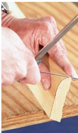
**3** **Angle the cut inward.** Start the cut with a few gentle pull strokes until the coping saw finds its groove; then switch to long push strokes.
