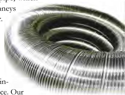
There is some discussion about whether rigid flue liners are easier to clean than flexible liners, which have a corrugated surface. Our most trusted expert says that flexible liners tend to collect less creosote when used to vent wood fireplaces and stoves because they flex as they expand and contract with temperature fluctuations, causing buildups to loosen and fall away.
