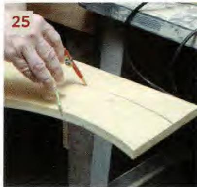
*Casing blank.* I use the curved jamb as a guide to lay out the inside edge of the curved blank on a sheet of MDF; then I rough-cut to the line with a jigsaw, and finish up the cut with a flush trim bit mounted in a router (23). To create the 1/4-inch reveal on the casing, I make one pass with a 1/4-inch rabbeting bit and a second pass with a flush trim bit (24).
