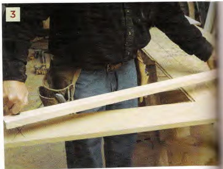
crosses the long layout line that indicates the base of the arch. Later on, I will transfer this mark to the back of the glue-up with a chisel so it doesn't get lost during sanding or routing. When I cut the trim, the mark will tell me exactly where the joint needs to be.
