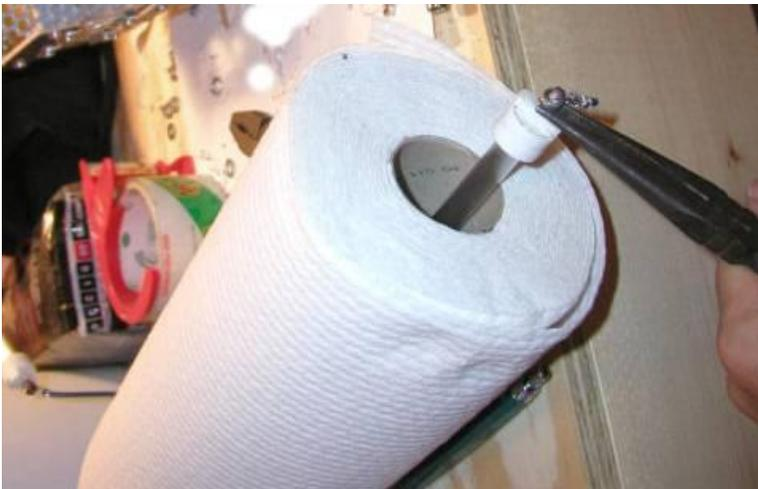
Here the rods have been installed. In order to do so, the metal holders at one end must be removed and the rod slid in from the end. Once an end of the rod is in place, the metal holders on the install end can be affixed over the rod. At that point the rods can be made parallel and a bit of free play in the rods can be insured.
