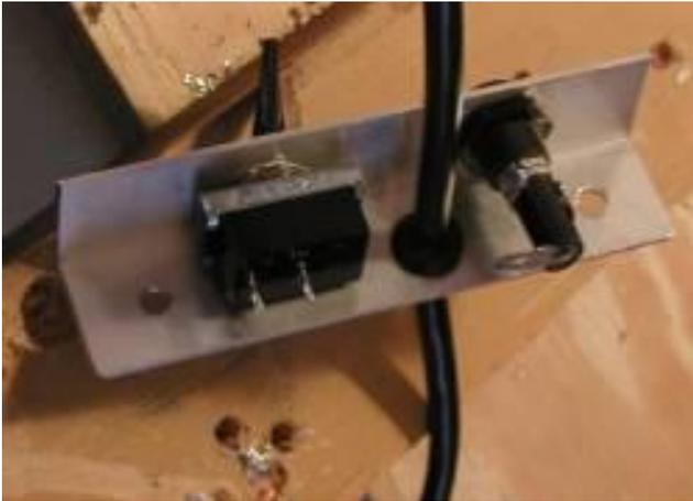
Here's my simple schematic. I re-used the wire from the heater, I figure it must be rated for heat in some regard. Connections to the quartz rods are via ring lugs crimped onto the wires. Connections to the switch and fuse are soldered although in retrospect that may not be so wise, I should replace them with quick disconnect lugs. Caution: your browser might size it down to fit the window:
