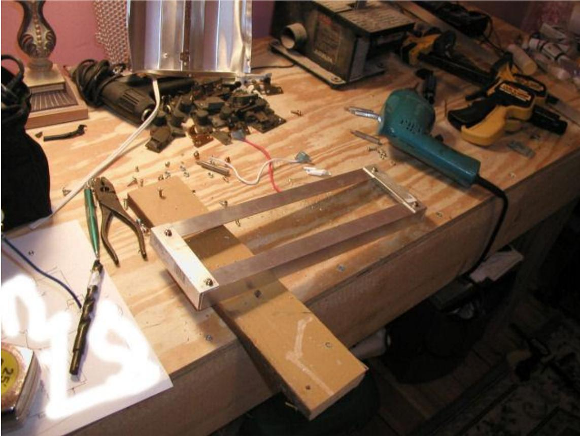
The "legs" of the IPR were next. I chose to make them 3.5 inches long. More screws, more washers, more nuts. Once the four legs were done I used 1"x1/8" aluminum (from Lowe's) for the "skirt". The image below shows me ready to cut it to length on the left. I ran the skirt "around" the base of the legs. In all it made a very strong box. It could support my weight without damage...
