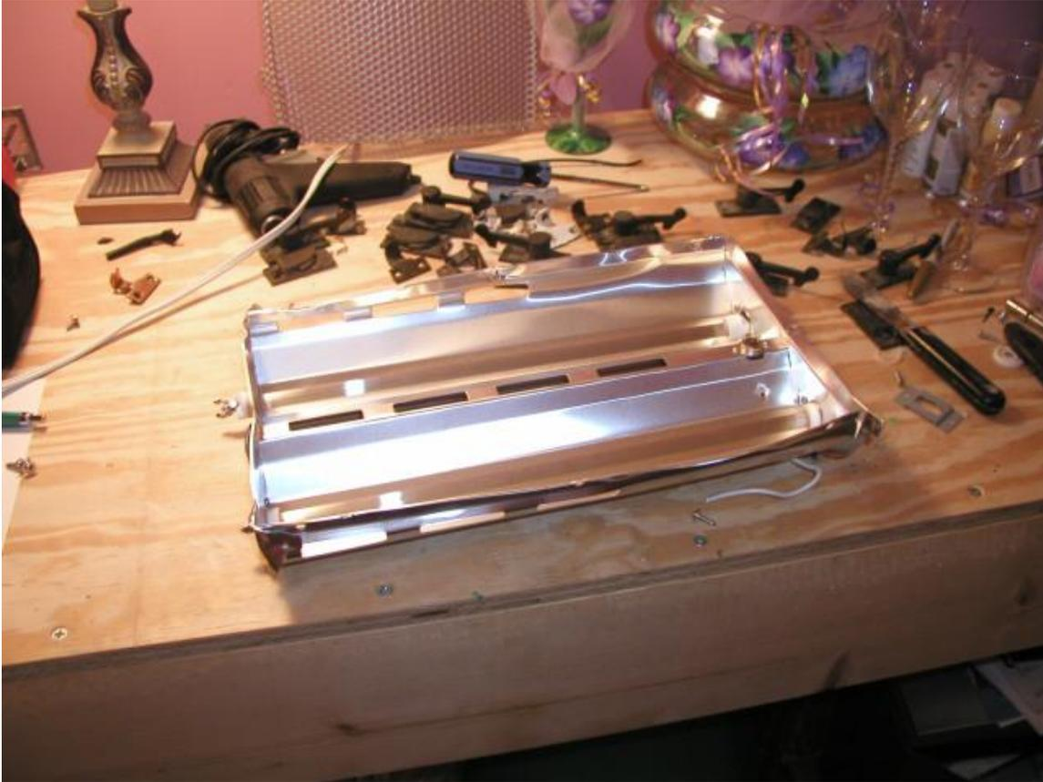
Now it was time to start constructing the box for the new IPR. I chose to use 1/8 inch angle aluminum from Lowe's. It would be easy to cut, not too heavy, same material as heaters are made from, strong, etc. I did my work with a hacksaw, you can make a smarter cut with a metal blade on a cut-off saw. I smoothed the edges and burs with a table sander...
